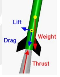
\*Center of Pressure – the point on the body about which the aerodynamic moment is zero.
